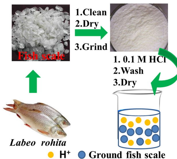
Fig. 1 Pathway of biosorbent preparation and activation by acid treatment
