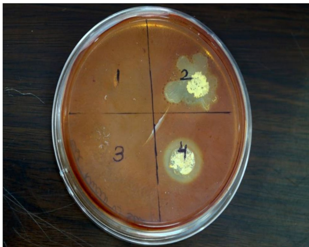
Fig. 11 Antibacterial activity of Starch (box 1); SGH-AgNPs against E. coli (box 2); SG-g-poly(AA) hydrogel (box 3) and SGH-AgNPs against S. aureus (box 4)
