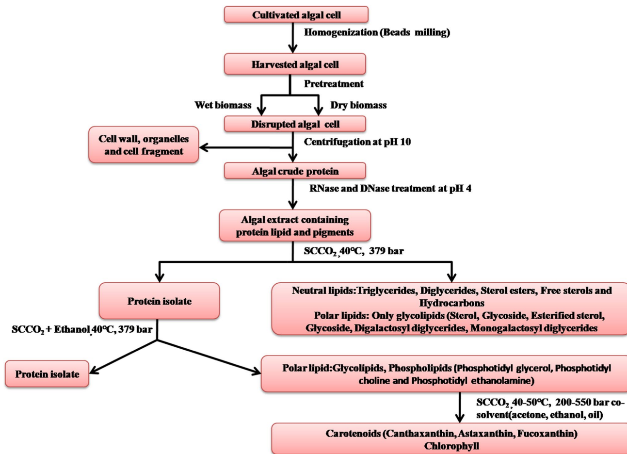
Fig. 3 Steps in the SCCO 2 extraction process for the extraction of different biomolecules from algae [29]
