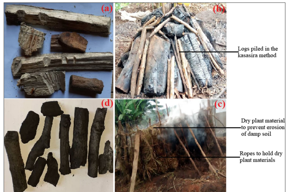
Fig. 1 Firewood (a); firewood piling (b); slow pyrolysis of firewood (c); and, developed charcoal (d)
