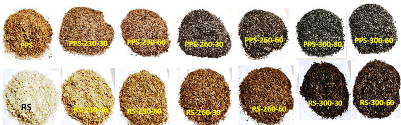
Fig. 2 Physical appearance of untorrefied and torrefied agro-wastes of palmyra palm shell (PPS) and redgram stalk (RS)
