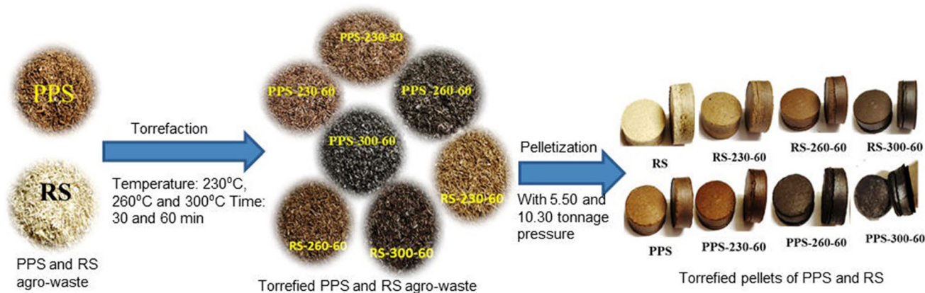
Fig. 1 Schematic route for the preparation of pellets from PPS and RS
