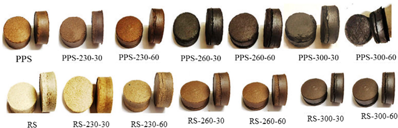
Fig. 9 Physical appearance of untorrefied and torrefied PPS and RS pellets with the change in temperature and time
