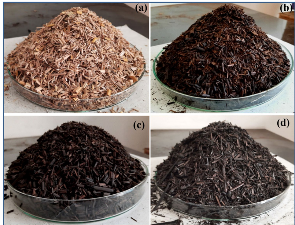
Fig. 2 Digital images of (a) as such rice straw and (b, c, d) rice straw torrefied at temperature 300 °C for different residence times of (b) 60, (c) 90, and (d) 120 min
