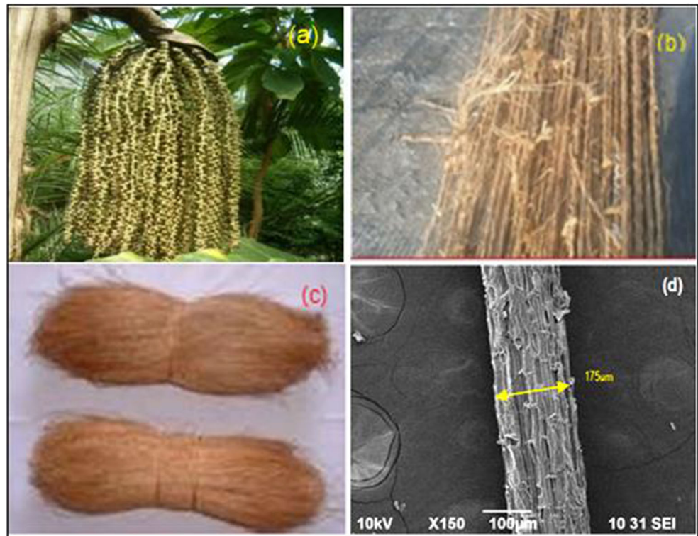
Fig. 1 Fibre extraction stages. (a) Fibre fruit, (b) fibre with sheath, (c) extracted fibre and (d) SEM image of a single fibre
