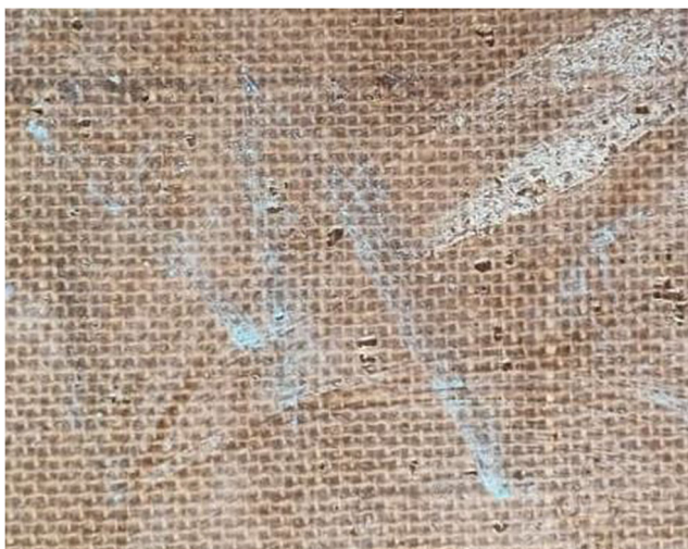
Fig. 5 Caryota fibre–reinforced epoxy composite
