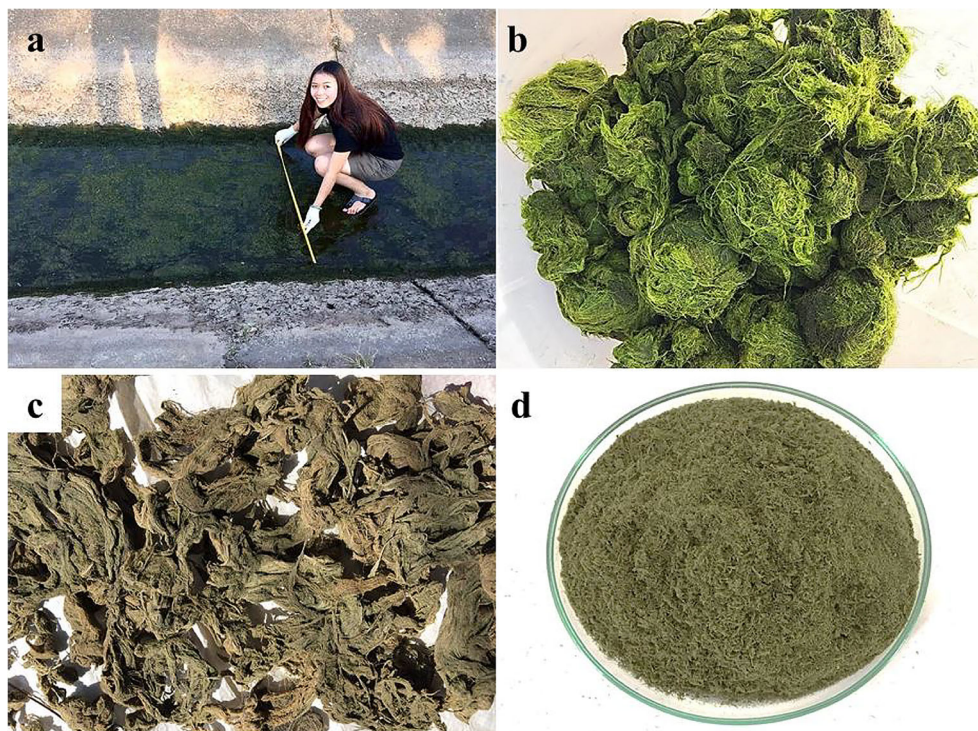
Fig. 1 (a) Sample collection of Rhizoclonium sp. in the canal (growing environment and sample), (b) harvested algae, (c) dried algae, and (d) powdered biomass
