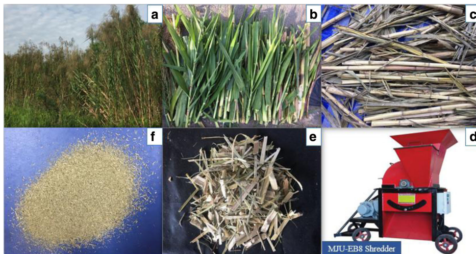
Fig. 1 Collection and preparation of material. a Grass field. b Cutting grass. c Dried grass. d Shredder machine. e Particle grass. f Grass powder
