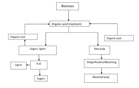
pulp was filtered off and washed with 80% fresh formic acid and finally with water. Pulp yield was determined gravimetrically on raw material. The kappa number of the resulting pulp was determined in accordance with Tappi test methods (T 236 om-99). All experiments were carried out thrice and average reading was taken.
