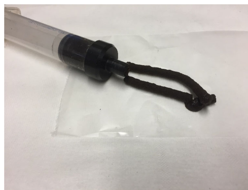
Fig. 2 The syringe test applied to an alkaline pretreated feed showing the homogeneity of the feed after the test
