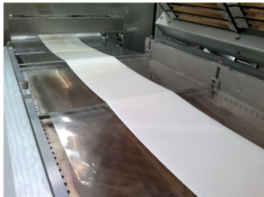
Fig. 5. A smooth layer of pigment-CNF dispersion was spread on top of the support material.
