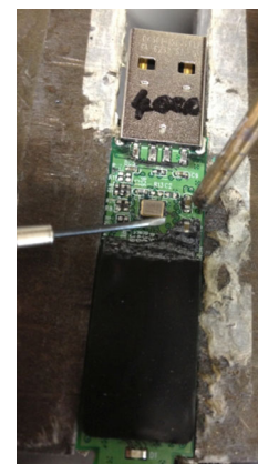
Fig. 3 Epoxy removal of Kingston DT 5000 with screwdriver
