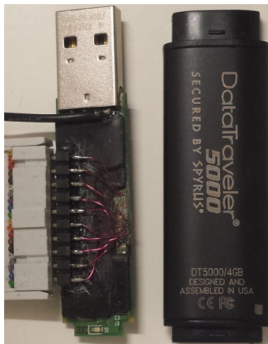
Fig. 4 Eavesdropping the bitstream of Kingston DT 5000 with opened case
