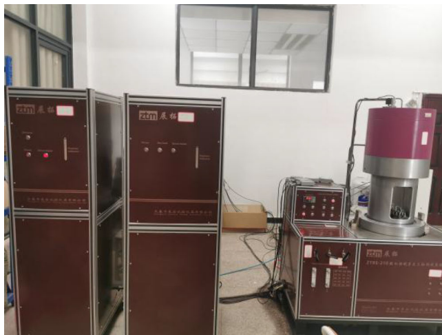
(a) Uniaxial loading system
