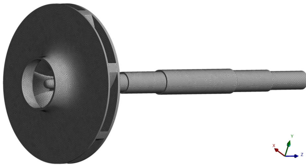
Fig. 7 The mesh of the solid domain
