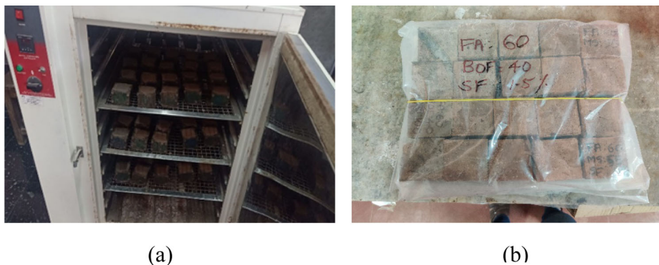
Fig. 7 a Oven curing b ambient cured samples
