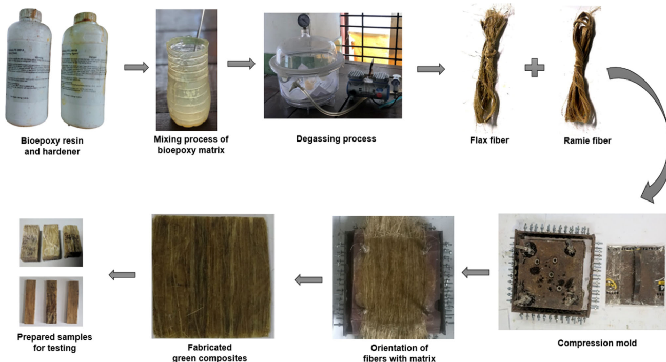
Fig. 1 Fabrication process of flax–ramie reinforced bioepoxy green composites
