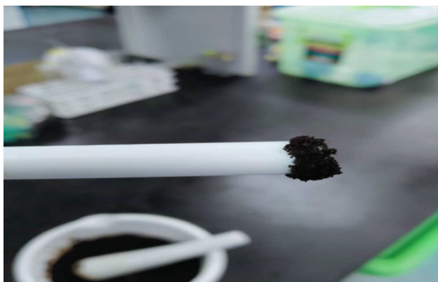
Fig. 9 Synthesized \text{Fe}_3\text{O}_4 -MNPs tested with laboratory magnet
