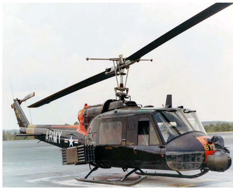
Fig. 5 UH1C “HUEY” helicopter (U.S. Army photograph from the official U.S. Department of the Army publication Vietnam Studies—Air mobility 1961–1971. Washington D.C. 1989)
