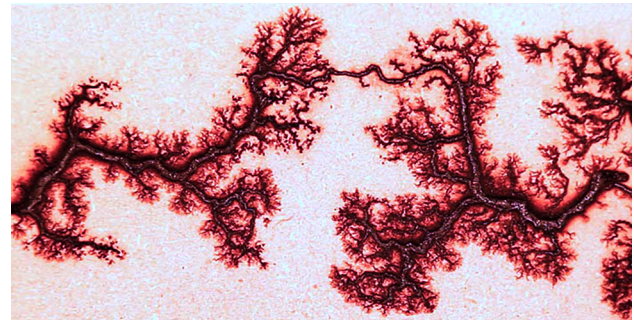
Fig. 2 Lichtenberg figure created on wood with high voltage electricity [46]
