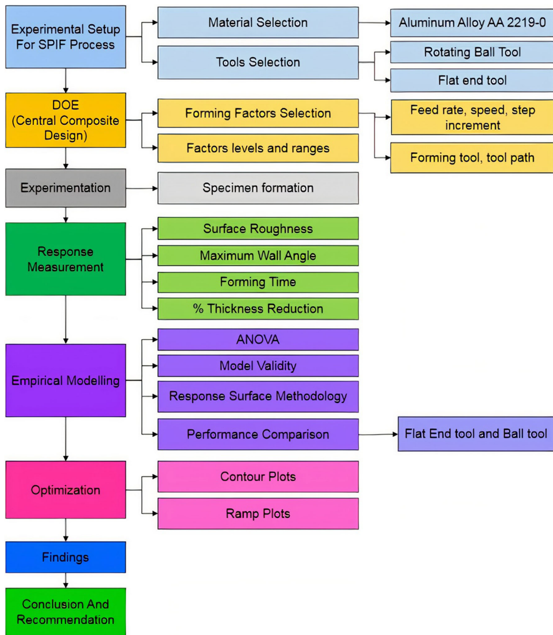
Fig. 1 Research methodology to evaluate the effect of critical SPIF parameters on the forming of Al alloy (AA2219-O)
