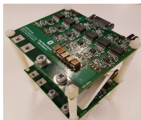
Fig. 17 Test setup: three-phase, three-port, five-level inverter
