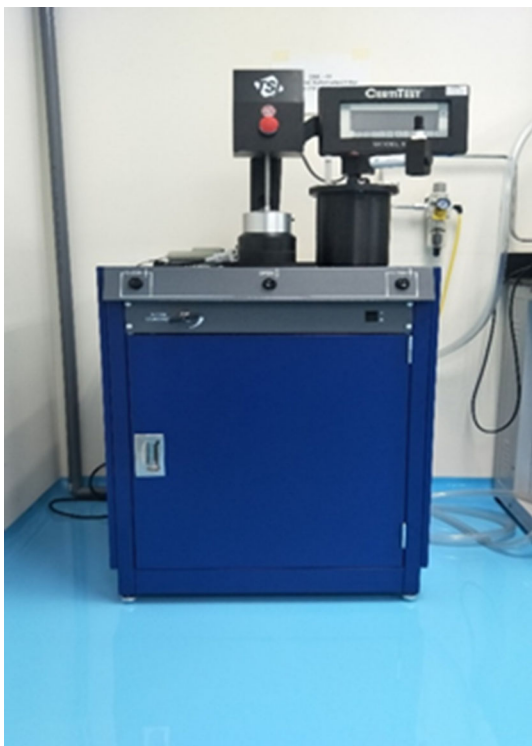
Fig. 3 Automated Filter Tester (TSI® Model 8130)
