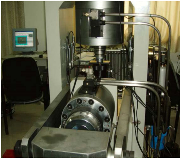
Fig. 12 The triaxial compression apparatus
