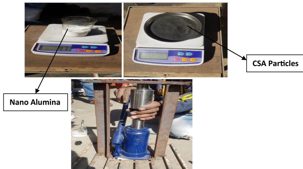
Fig.3 Preparation of powder (Pure Al + nano-alumina)
