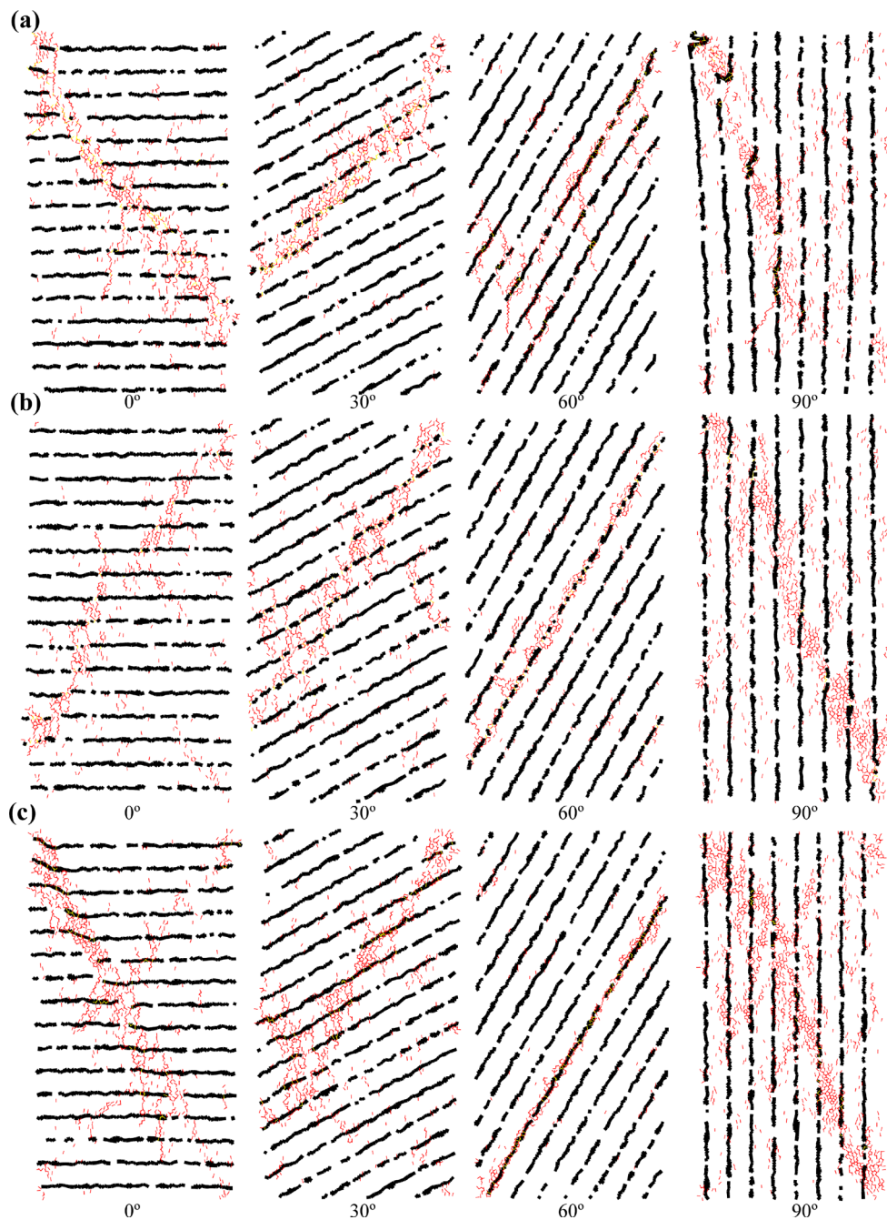
Fig. 11 Failure mode of phyllite under PFC. a Dry; b Watery; c Saturated water
