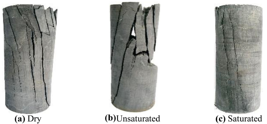
Fig. 8 Failure modes of different layers of phyllite. a Dry condition (0%); b Unsaturated condition (1.5%); c Saturated condition (2.7%)
