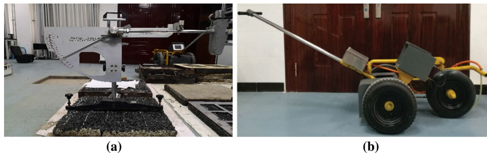
Fig. 4 Test devices for evaluation of antifreezing performance: a British pendulum tester, b walking frictional tester
