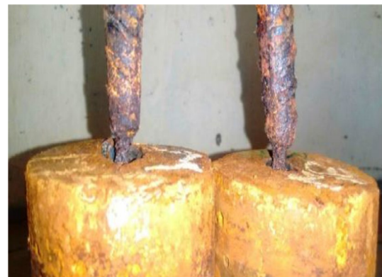
Fig. 16 Specimens after testing DA0 (DA0=CC; i.e., without inhibitor addition)
