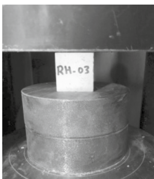
Fig. 3 Compressive strength test using the universal testing machine
