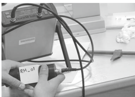
Fig. 4 Testing P-wave velocity using Proceq Pundit Lab+UPV Instrument
