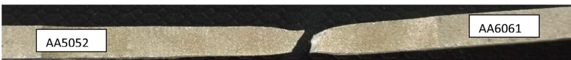
Fig. 11 a Stress–strain curve for optimal parameter combinations (trial 6). b Weld profile for the optimal parameter combinations. c Fractured specimen for the optimal parameter combinations
