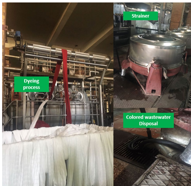
Fig. 1 Real photographs from the factory representing the dyeing process with the colored wastewater disposal
