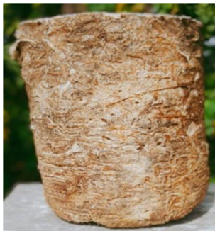
Fig. 3 Mycelium-sawdust composite samples
