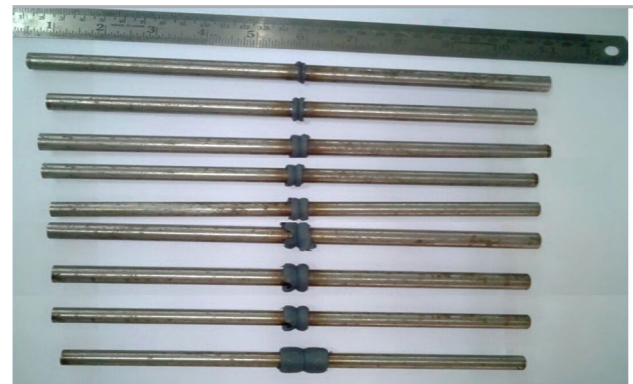
Fig. 3 Sample joints formed during friction welding
