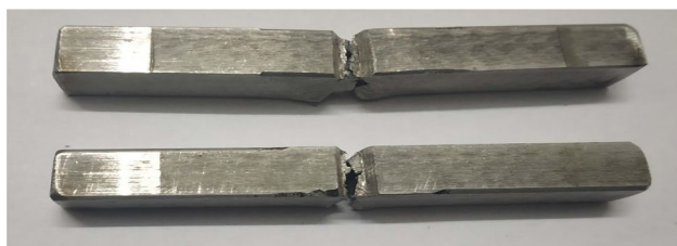
Fig. 7 Specimen subjected to Charpy V-notch test
