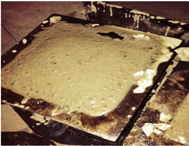
Fig. 7 Gas formation in AF mix
