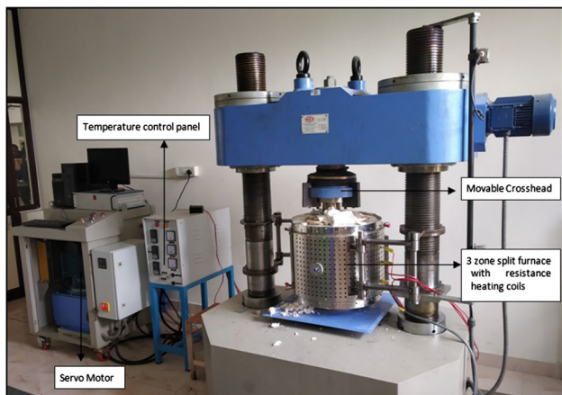
Fig. 5 Compression machine used for V-bending
