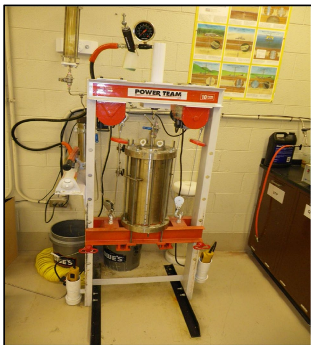
Fig. 9 Impermeable and permeable fracture tester
