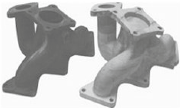
Fig. 2 Gray iron casting using sand mould [3]
