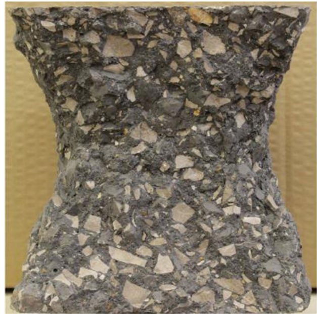
Fig. 4 Compressive failure of concrete specimen with w/c of 0.35 and 0.05% CNTPL
