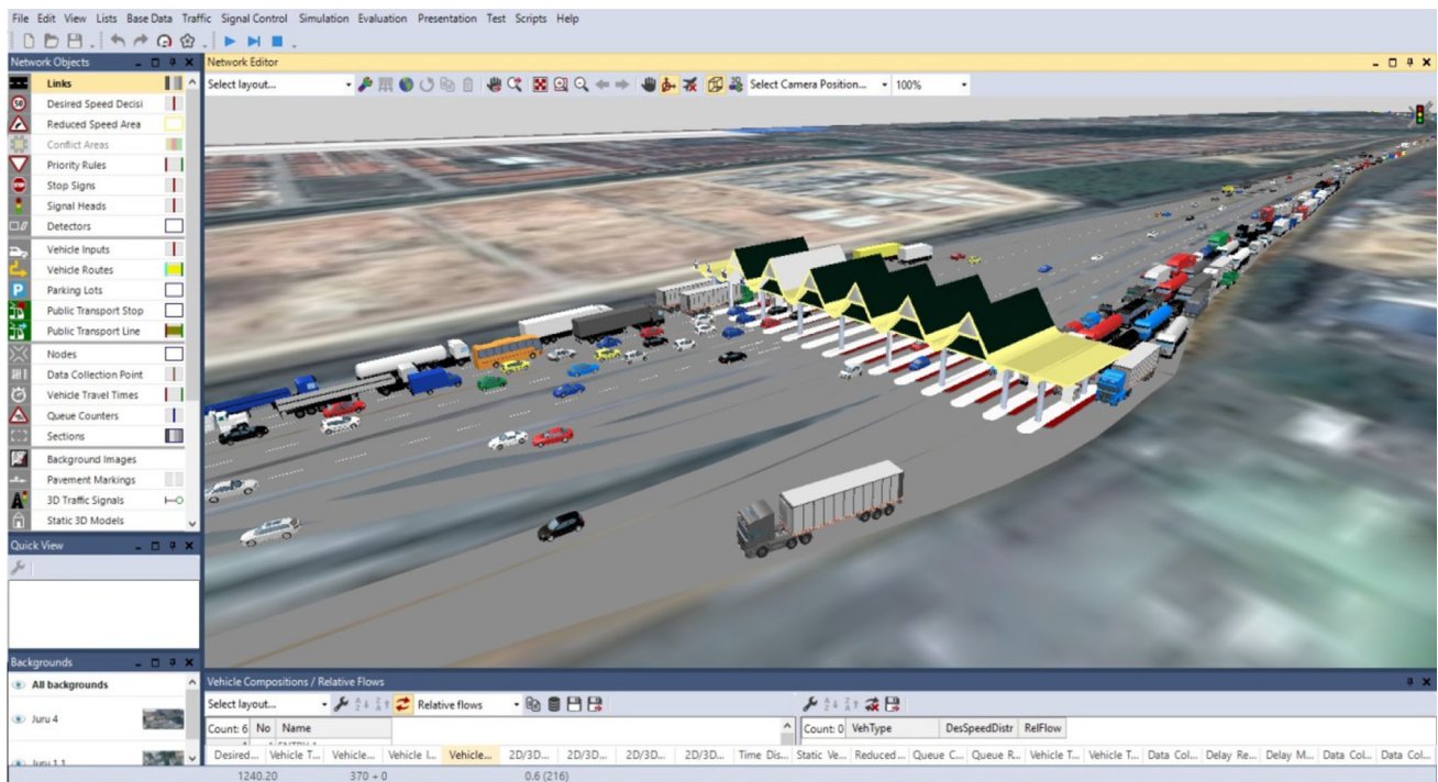
Fig. 15 Screen-captured image of the 3D simulation model of Juru toll plaza
