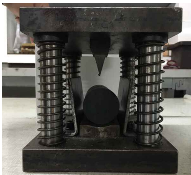
Fig. 2 Photograph of the custom-made shale splitting device with a specimen ready for splitting
