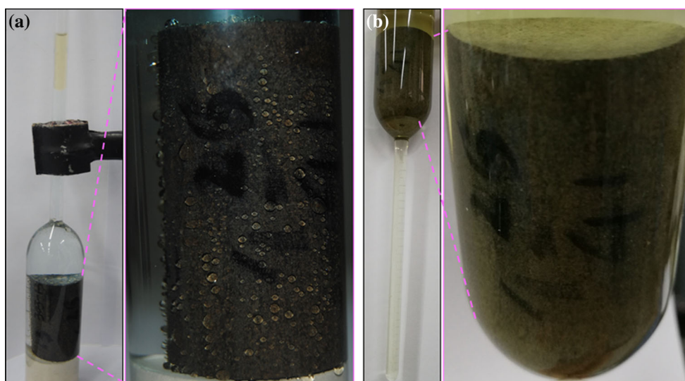
Fig. 2 a Oil droplets at the surface of the cylindrical core plug during spontaneous imbibition experiment in water; b core plug spontaneous imbibition in oil
