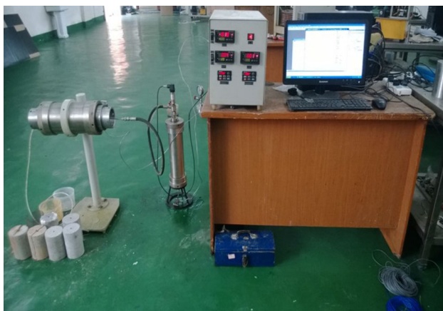
Fig. 12 Experiment apparatus of pressure-bearing capacity
