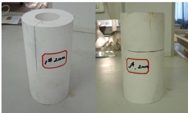
Fig. 8 Cylindrical artificial cores with fracture
