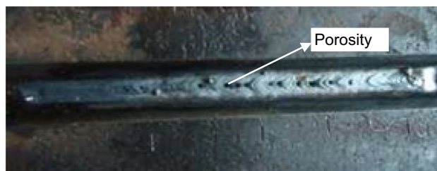
Fig. 11 Resultant weld with porosity (Grease)
