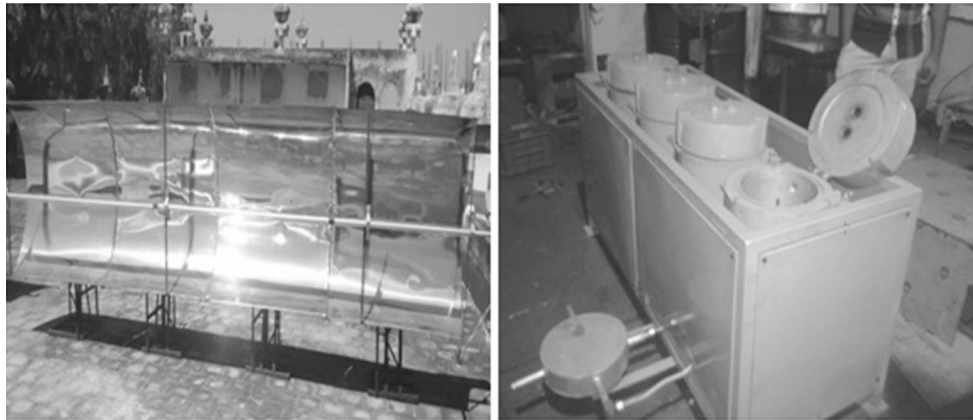
Fig. 2 Photographic view of PTC and Cascaded TES system
