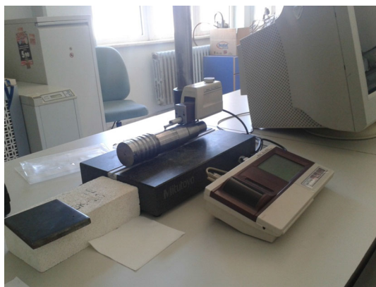
Fig. 5 Experimental set-up for surface roughness measurement
