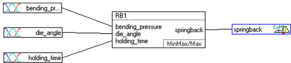
Fig. 12 Structure of the fuzzy logic system
