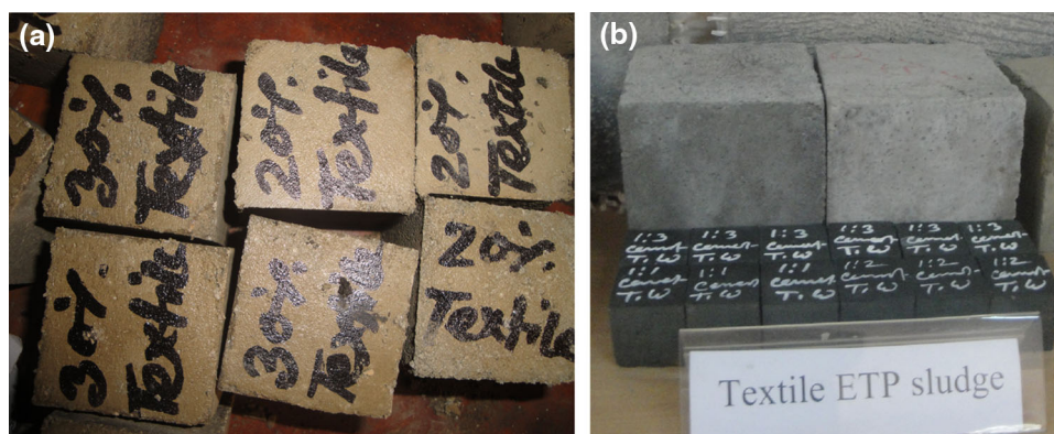
Fig. 2 Test sample: a mortar specimens containing Portland cement, sand and ETP sludge at the ratio of 1:3.76:0.25, b mortar and concrete specimens with varying sludge content
