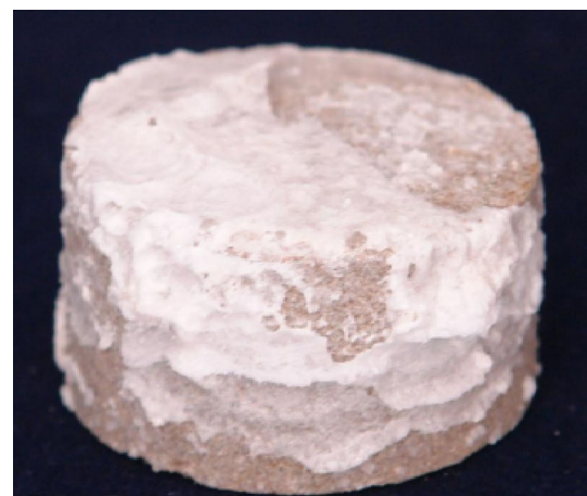
Fig. 8 Sandstone sample used in static adsorption test of DSNP solution
