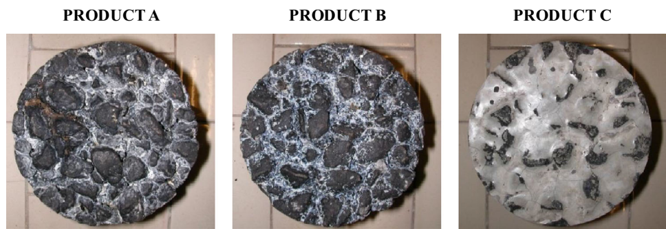
Fig. 3 Core pictures for white pixel percentage analysis
