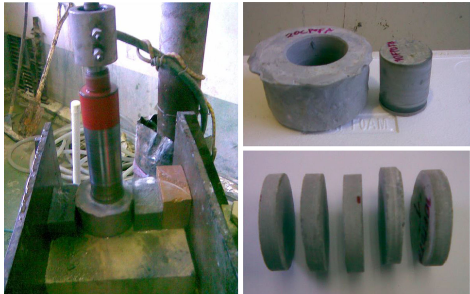
Fig. 2 Paste specimens coring and cutting for chloride test
